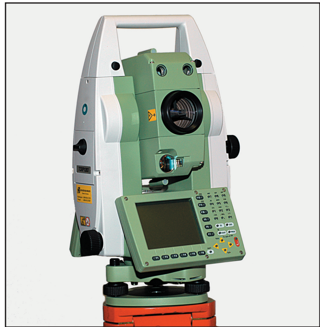
Figure 2— A commercial total station used for surveying (instrument provided for this study by Selby's Engineers Service and Supply Co., Missoula, MT).
