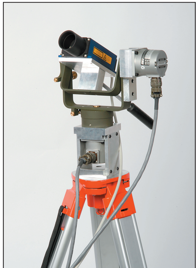
Figure 1—The prototype MTDC laser surveying station (the laptop computer and the box with the electronic interface to the laptop are not shown).
