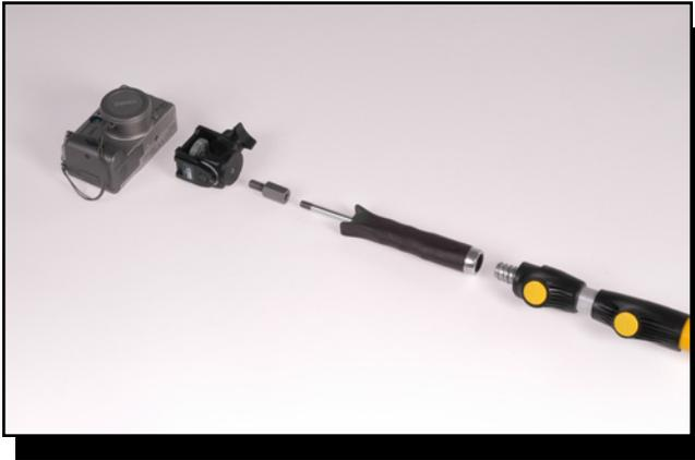
Figure 10—Detailed view of the camera-with-altitude unit using a paint pole rather than a monopod and hiking staffs.
