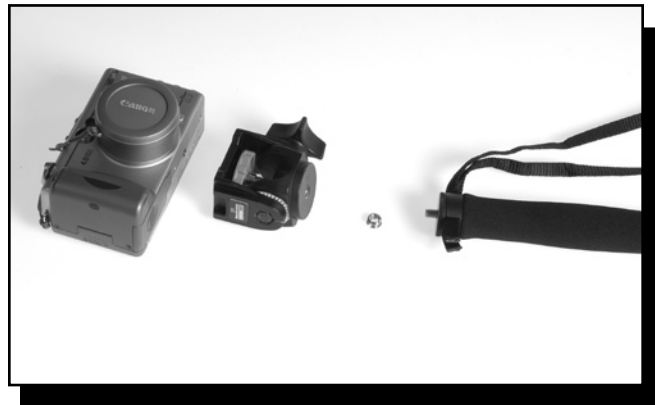
Figure 8—A bushing converts the hiking staff's \frac{1}{4} -in mount to a \frac{3}{8} -in mount for the Bogen tilt head.
