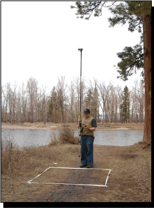
Figure 3—Hiking staffs specially configured to support a camera with altitude for site monitoring.
