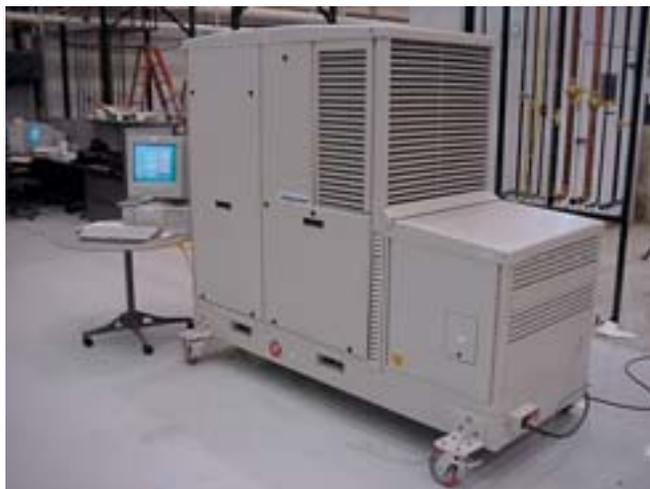
**Figure 2.** *This 5-kilowatt fuel cell manufactured by Plug Power is being tested by the U.S. Department of Defense at the Concurrent Technologies Corp. test facility. It is intended for residential use or small commercial installations. —Photo courtesy of Concurrent Technologies Corp., Johnstown, PA.*
