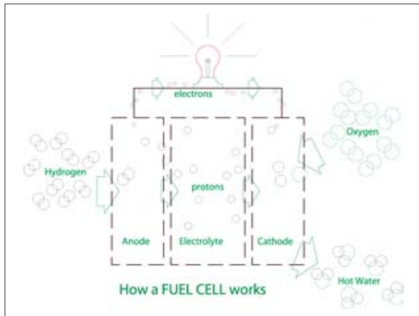
**Figure 1.** This schematic drawing shows how fuel cells produce electricity.
