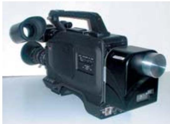
**Figure 3.** *The black box (foreground) attached to this commercial video camera is a fuel cell manufactured by Jadoo Power Systems. The fuel cell replaces much heavier batteries and is used whenever a portable power source is needed. —Photo courtesy of Jadoo Power Systems, Folsom, CA.*
