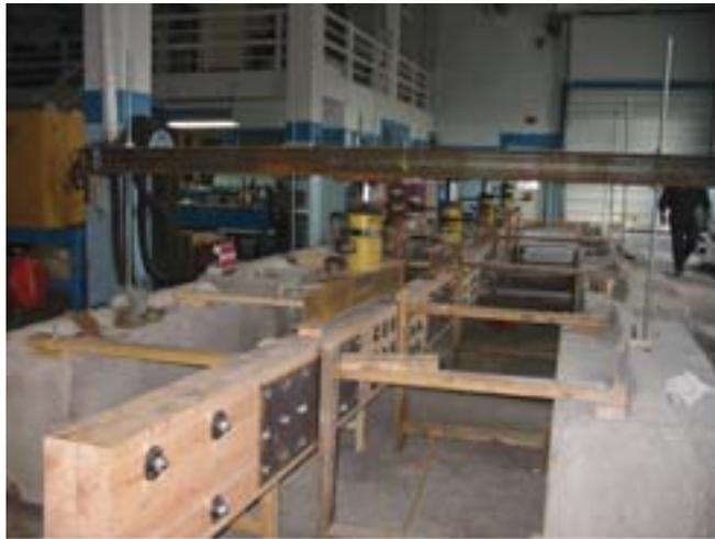
**Figure 8.** *Staggered stringer load test.*
