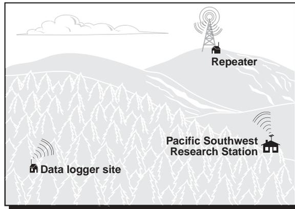
The research station had access to a VHF repeater maintained by the Sierra National Forest. One channel on the repeater received very little use. The research station's data could be downloaded during the early morning hours using that channel. A modem from Teledesign Systems of San Jose, CA, solved the problem of shipping data over a channel designed for voice communication. This modem
