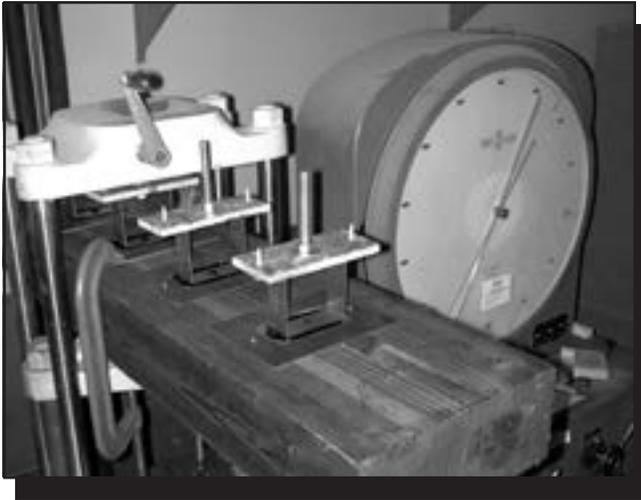
Figure 17—Testing the tensile strength of asphalt adhesion.
