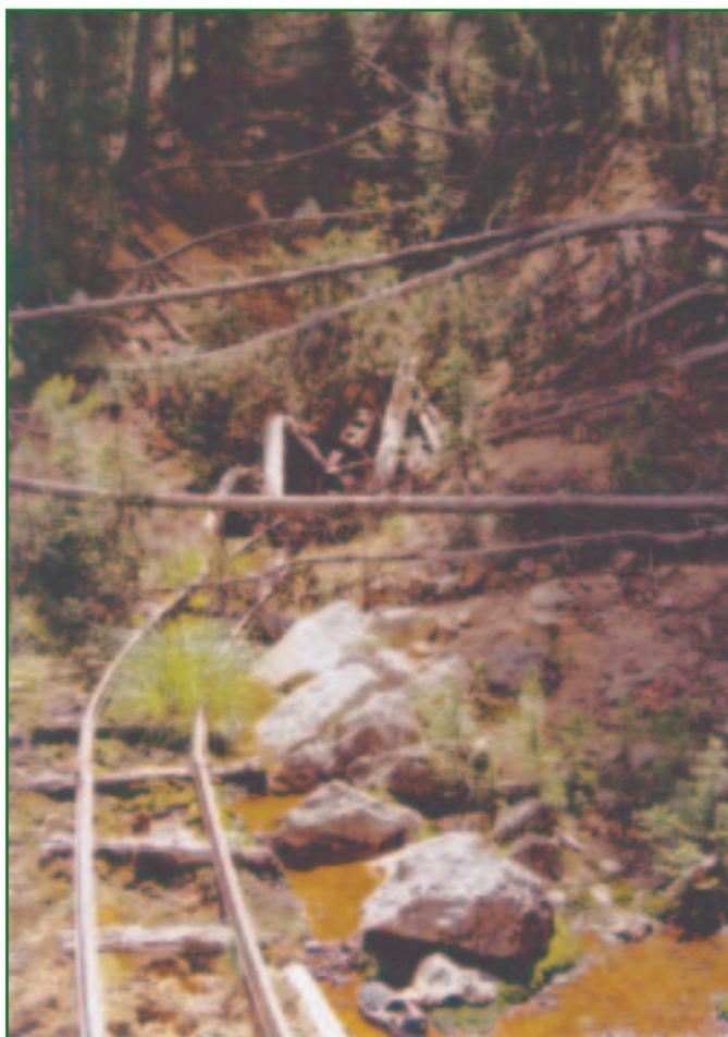
Figure 8—Looking upslope into collapsed hillside mine workings about  $\frac{3}{4}$  mile south of the Elkhorn Mine upper adit. A small, very acidic flow (pH 4.2) emerges from the workings, then becomes groundwater 30 feet downstream. The water deposits thick iron coatings on soil and rocks in the shallow channel.
