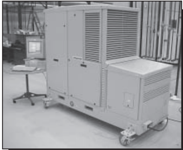
Figure 5—This 5-kilowatt fuel cell manufactured by Plug Power is being tested by the U.S. Department of Defense at the Concurrent Technologies Corp. test facility. It is intended for residential use or small commercial installations. —Photo courtesy of Concurrent Technologies Corp., Johnstown, PA.
