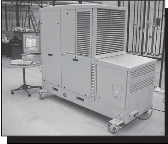
Figure 5—This 5-kilowatt fuel cell manufactured by Plug Power is being tested by the U.S. Department of Defense at the Concurrent Technologies Corp. test facility. It is intended for residential use or small commercial installations. —Photo courtesy of Concurrent Technologies Corp., Johnstown, PA.
