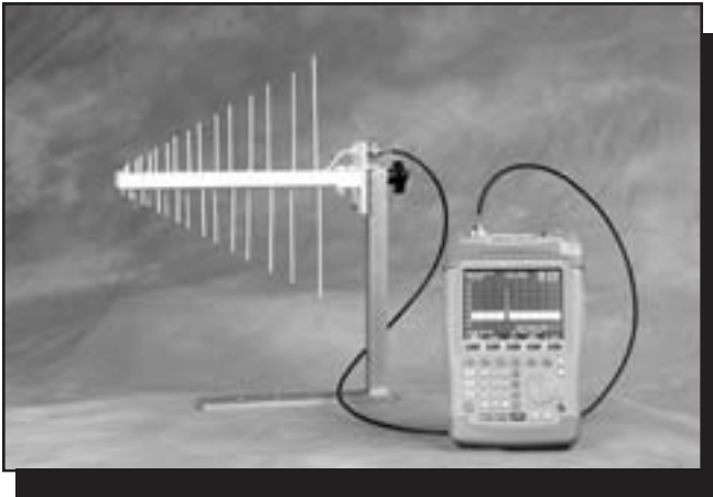
Figure 2—The log periodic Yagi antenna (left) and a spectrum analyzer were used to determine signal strength from the UHF Motorola hand-held radio.
