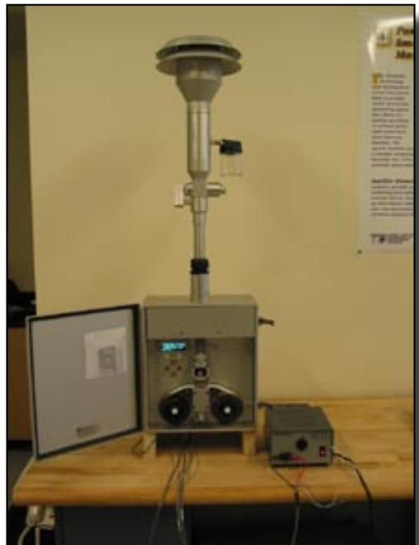
Figure 3—The E-BAM monitor with its environmental door open. The instrument collects particulate on a filter tape that automatically advances when the tape is full.
