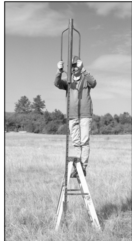
Figure 2—Standard fence post drivers require the operator to stand on a ladder or raised platform to drive a 10-foot-long metal T-post.
