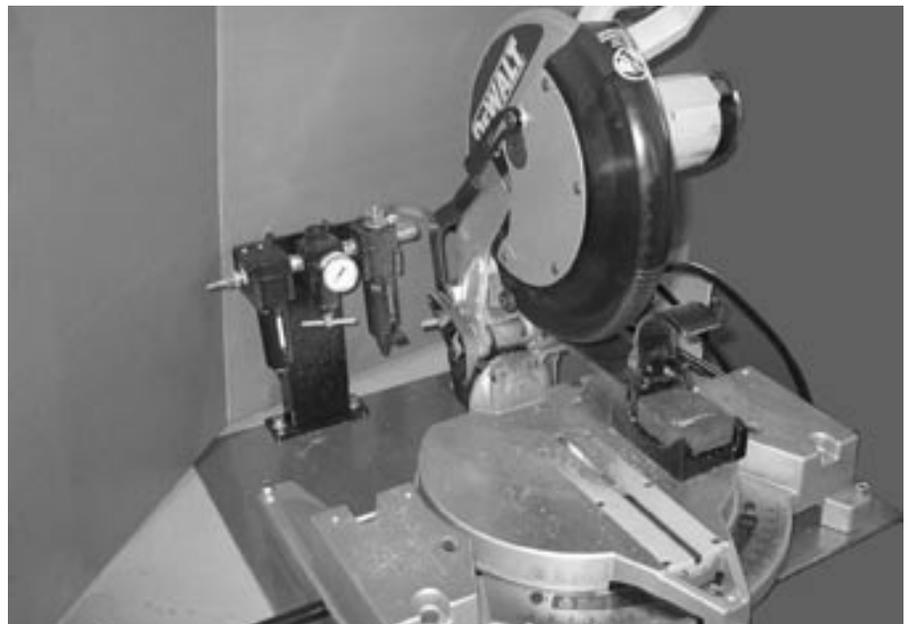
Figure 1—The power miter saw (DeWALT DW705) was modified to cut hardwood whips for planting.
