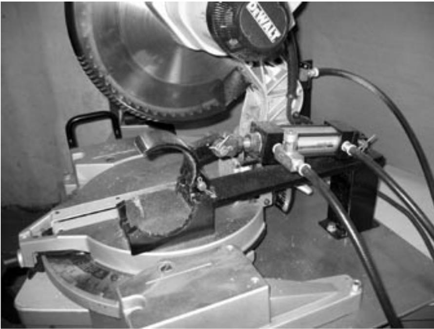
Figure 2—This pneumatic clamp secures the whips so they can be cut safely.
