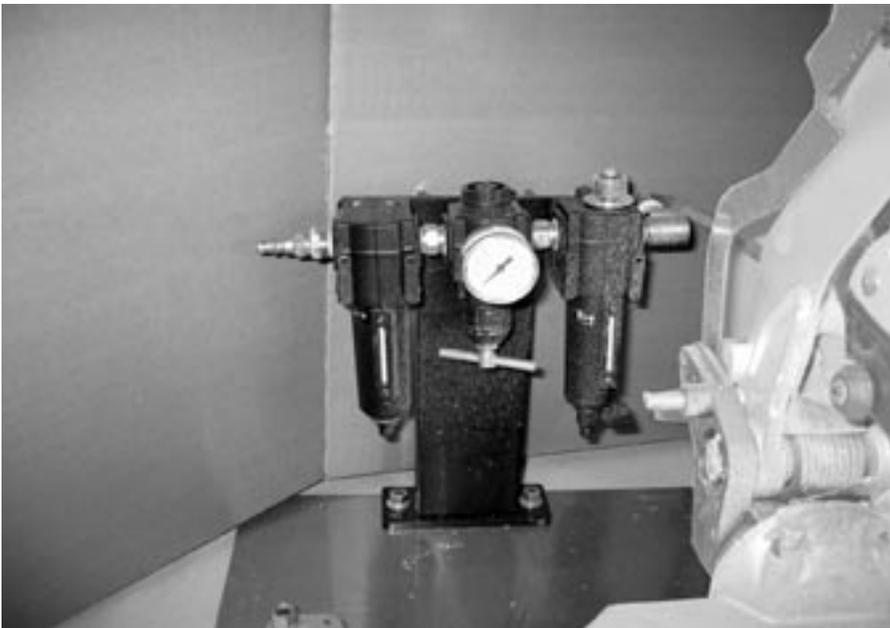
Figure 3—The source of compressed air includes a filter, pressure regulator, and lubricator.
