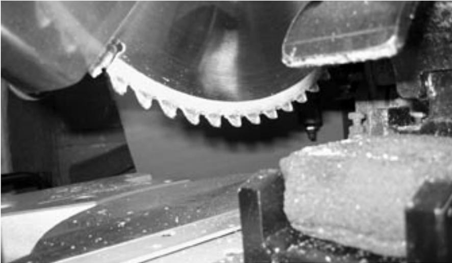
Figure 7—The 60-tooth saw blade was covered with sap after 2 weeks of use, but it still worked well.
