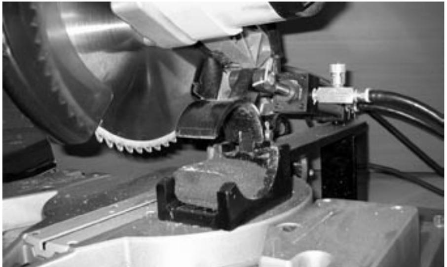
Figure 5—A rigid foam pad inside the clamp helps secure different sizes and shapes of whip bundles.
