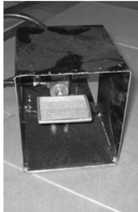
Figure 4—A foot-operated pneumatic valve activates the clamp.
