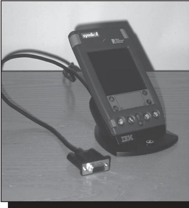
Personal digital assistant configured for bar-code scanning with the docking terminal and cable system.
