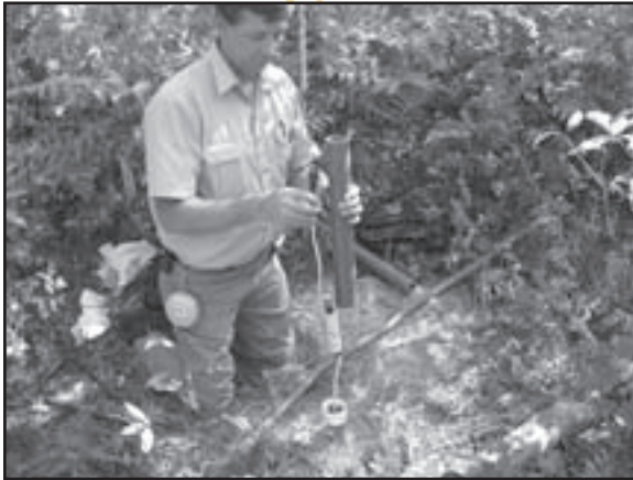
An electronic water table logger helps provide more frequent and more accurate water table data.
