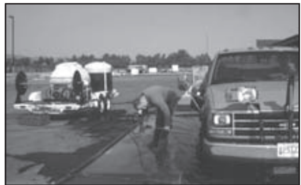
Portable vehicle-washing systems will reduce the amount of weed seed and other undesirable material spread by vehicles operating on Forest Service roads.
