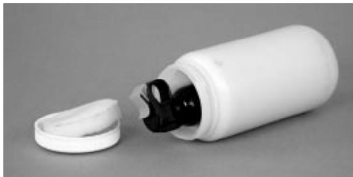
*The recommended storage container is a simple Nalgene plastic bottle lined with open-cell furniture foam. The foam traps the active ingredient while allowing the propellant to escape.*
