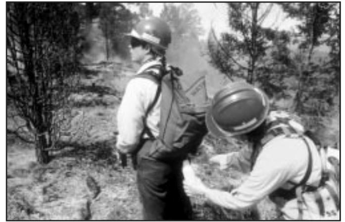
*The center developed nylon fabric water bags with replaceable plastic liners to assure that drinking water was sanitary. The bags are available in different sizes for carrying on a firefighter's back, in a truck, or slung beneath a helicopter.*
