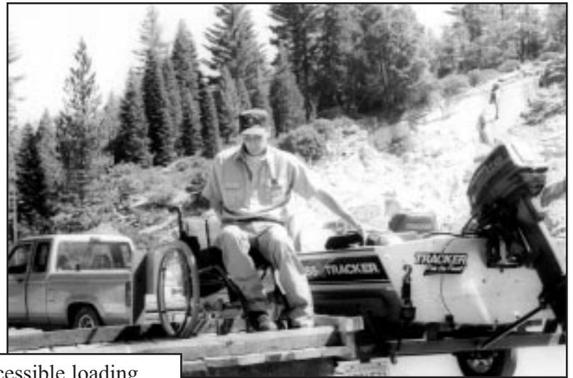
Accessible loading platforms make it easier for people with limited mobility to get in and out of boats. Once boaters have boarded, the boat is backed to the water for launching. This platform and drawings were developed by the center.
