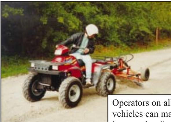
Operators on all-terrain vehicles can maintain lanes and trails using accessories developed by the center.
