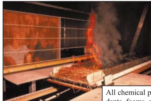
All chemical products (such as retardants, foams, and gels) for wildland firefighting must be proven safe and effective before the Forest Service qualifies them for use. This wind tunnel test of the effectiveness of fire retardant is one of many tests the center conducts on each product.
