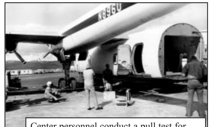
Center personnel conduct a pull test for the Federal Aviation Administration during the 1980s. This test shows that the center's anchor for parachute static lines can safely handle anticipated loads. Nearly every smokejumper aircraft used by the Forest Service has been equipped with modifications designed by the center.
