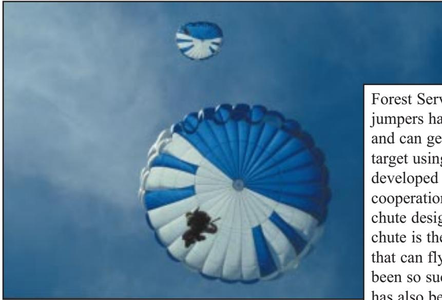
Forest Service smoke-jumpers have softer landings and can get closer to their target using a new parachute developed by the center in cooperation with a parachute design firm. The parachute is the first round chute that can fly backward. It has been so successful that it has also been adopted by the U.S. Army.
