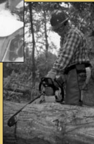
*Kevlar fabric in chain saw chaps protects users from injuries. The chaps were developed during the 1960s. Testing devices make sure that the chaps continue to work even as chain saws are improved.*
