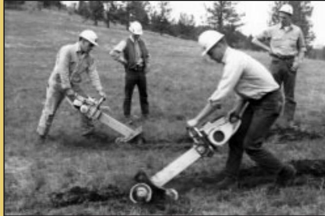
This modified chain saw is one of many tools the center has evaluated for building fireline. Although the tools were fast, they threw rocks and posed other safety hazards.
