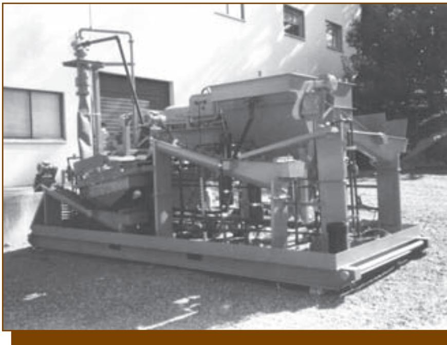
Figure 13—Typical soil washing unit.
