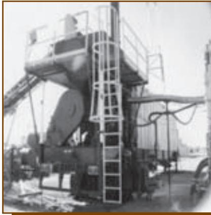
Figure 12a—Two views of a typical portable thermal desorption unit.
