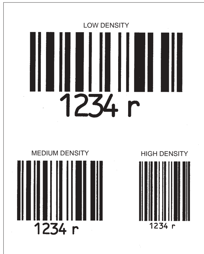
Figure 2—Bar-code density is one of the factors that determine the size of the bar-code label you should use.
