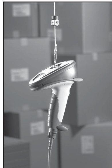
Figure 3—This scanner is attached to a pulley with a steel cable. The scanner can be moved in the storage area, but is less likely to be lost or damaged.
