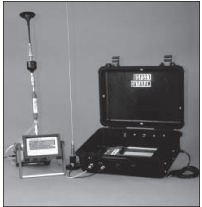
Figure 6—DataRAM4 connected to the telemetry unit.
