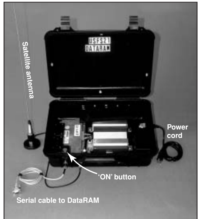
Figure 5—Remote telemetry unit used with the DataRAM4.
