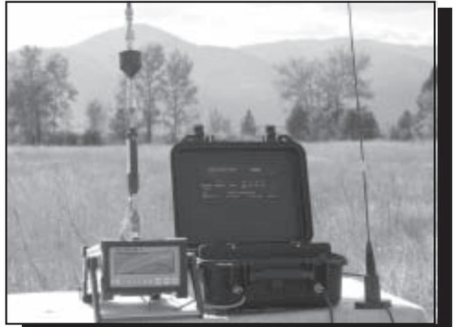
Figure 3—The AQD4-2000 MK II telemetry system.
