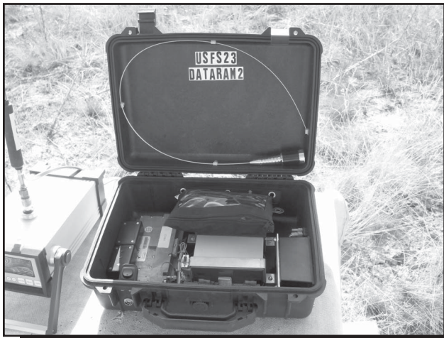
Figure 2—A DataRam particulate monitor and the AQD4-2000 remote telemetry system.
