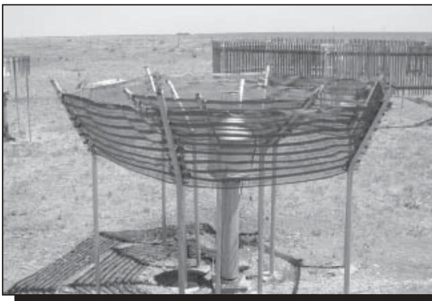
Figure 4—The catch efficiency for the half-scale Wyoming windshield drops rapidly as wind increases.
