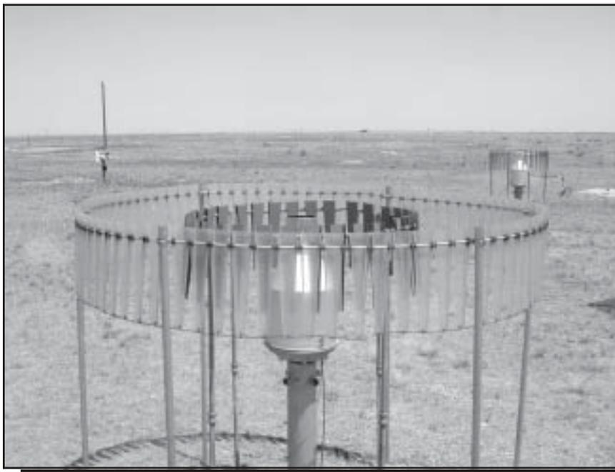
Figure 3—The double Alter windshield performs well in high winds.
