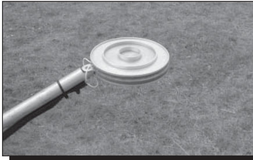
Figure 5—The hotplate snow gauge does not require a windshield.
