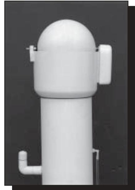
Figure 6—This Canadian rotating ball gauge does not require a windshield.
