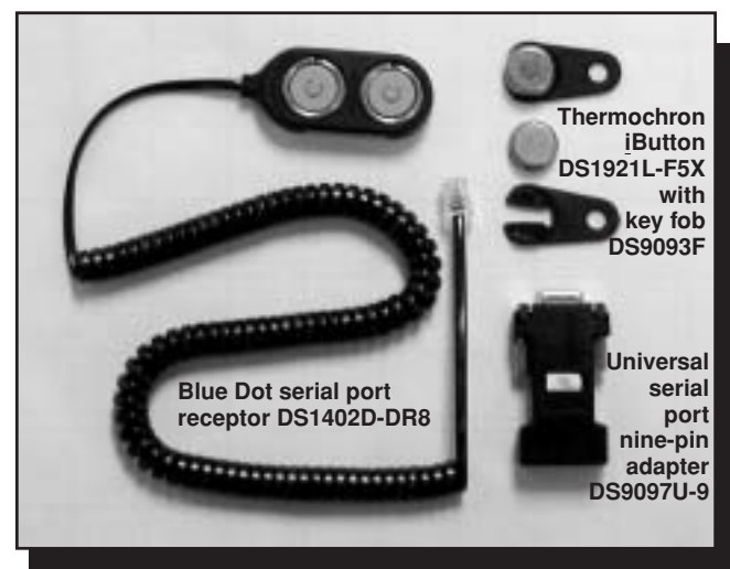
Figure 1—The Thermochron iButton data logger with hardware that allows it to communicate with an IBM-compatible computer.
