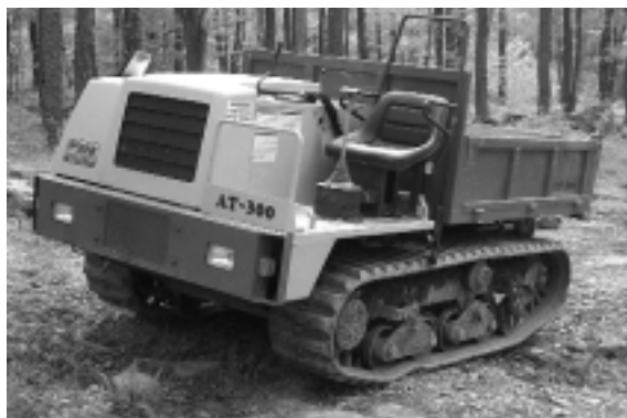
Figure 2. A minitracked trail dumper.
