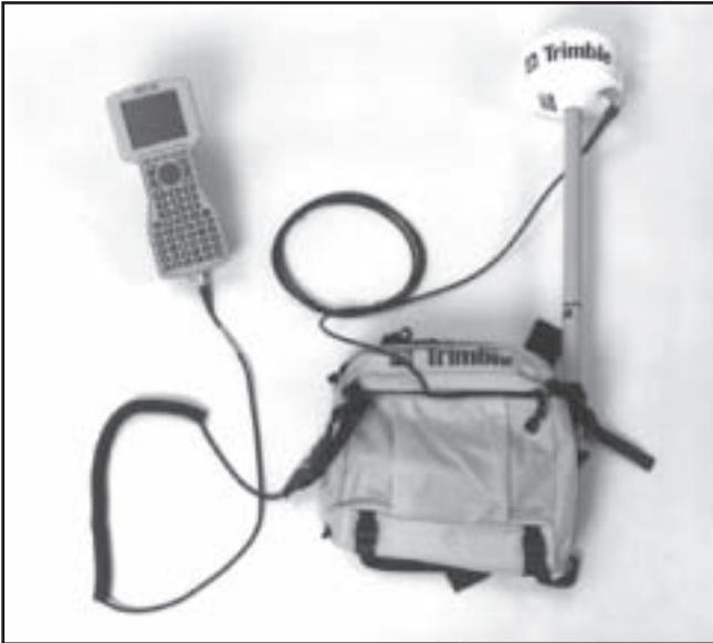
Figure 7—Trimble Pro XR GPS receiver.
