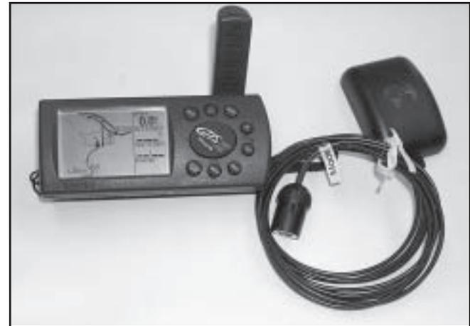
Figure 6—Garmin GPS III+ receiver.
