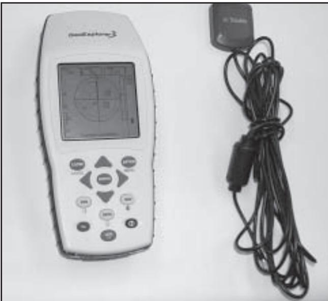
Figure 8—Trimble GeoExplorer 3 GPS receiver.
