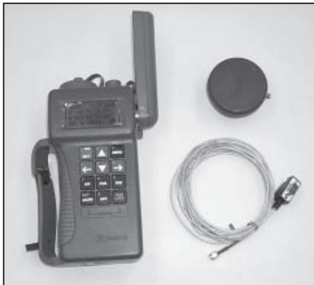
Figure 5—Rockwell PLGR +96 P(Y) code receiver.
