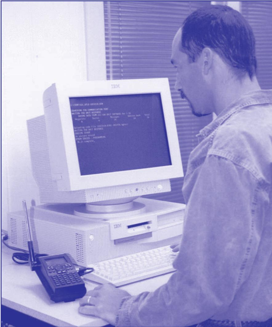
Figure 2—Updating the GSC-100 software using an IBM-compatible computer.
