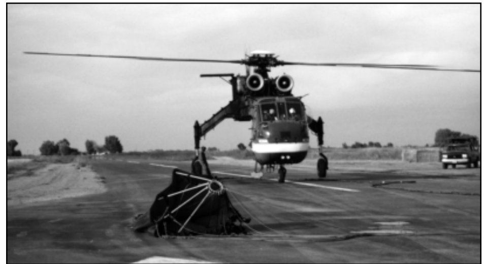
Figure 1—The Siller Brothers S-64 with 2,000-gallon Bambi helibucket.
