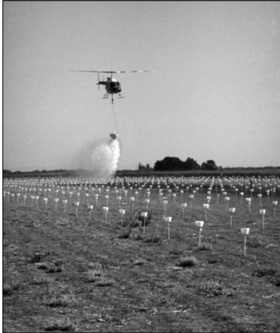
Figure 4—Drop test of the Forest Service Bell 206 with 100-gallon Sims helibucket using water.
