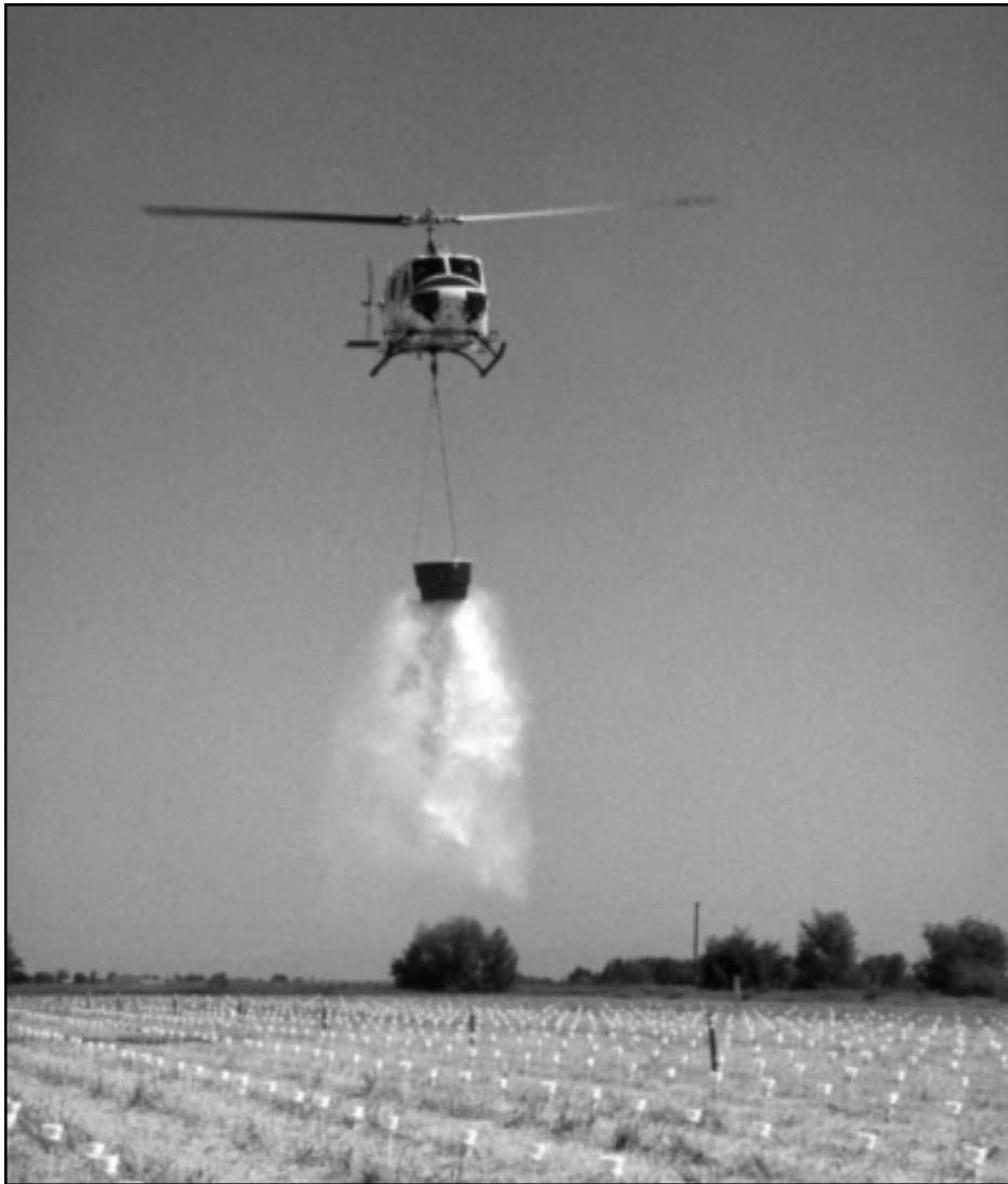
Figure 8—Drop test of the CDF Bell S205 with 300-gallon Sims collapsible helibucket using water.
