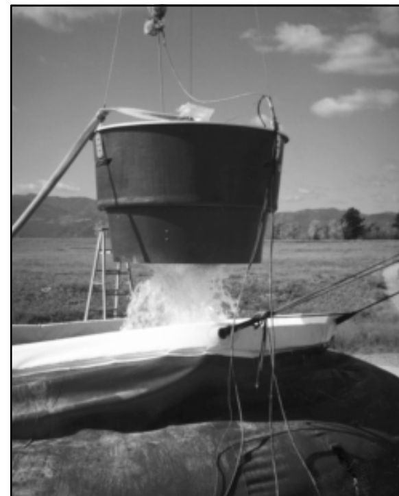
Figure 1—A static test of the 300-gallon Sims collapsible helibucket.
