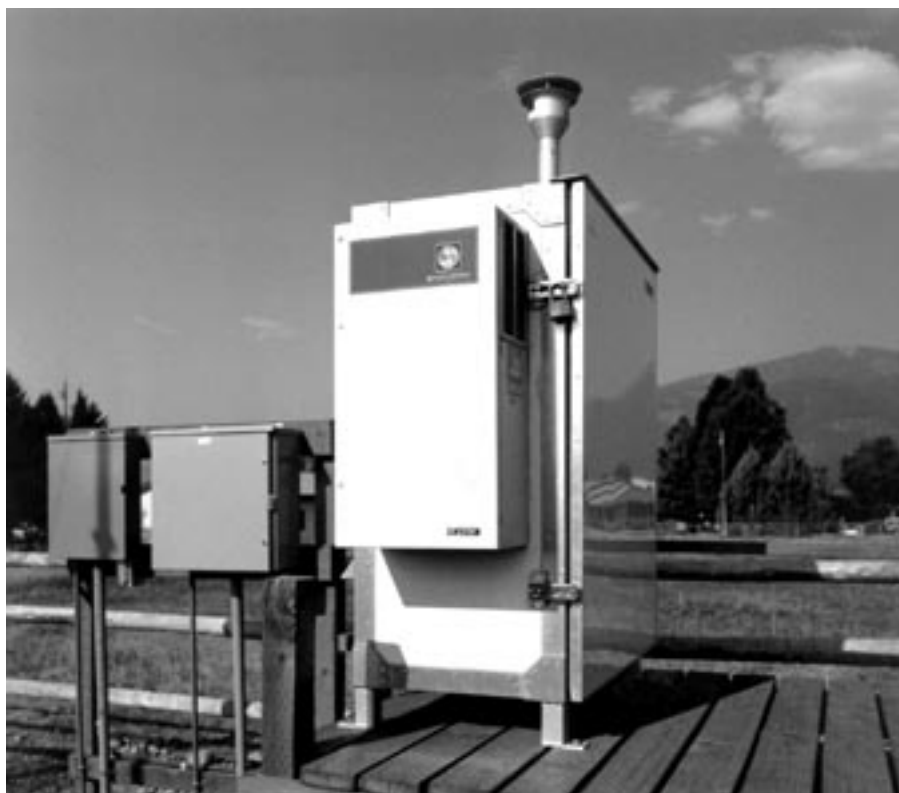
Figure 14—The Rupprecht & Patashnick tapered element oscillating microbalance instrument.
