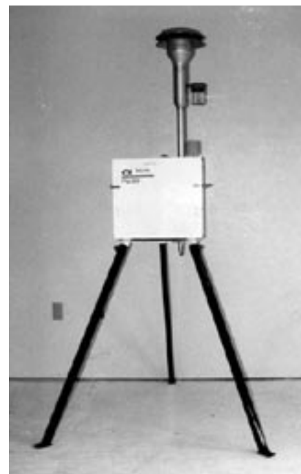
Figure 15—The BGI PQ 200 federal reference method PM 2.5 air sampler.
