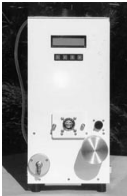
Figure 11—The Optec NGN-3 PM_{2.5} size-cut nephelometer
