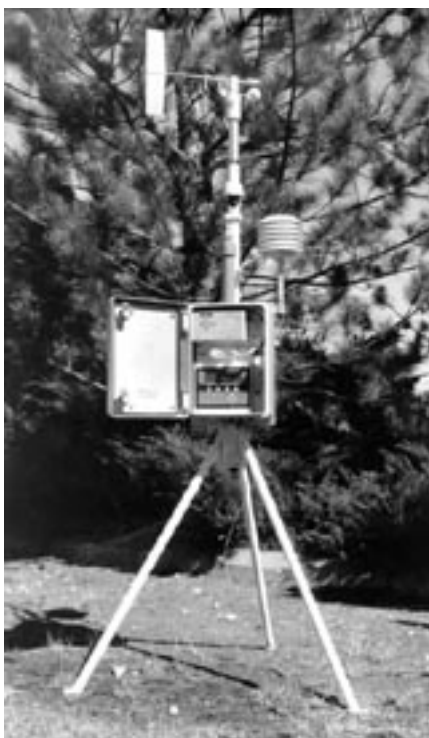
Figure 9—The Met One GT-640 particulate monitor with meteorological instrumentation.
