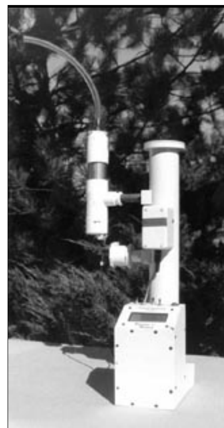
Figure 12—The Radiance Research M903 nephelometer (with attached inlet heater).
