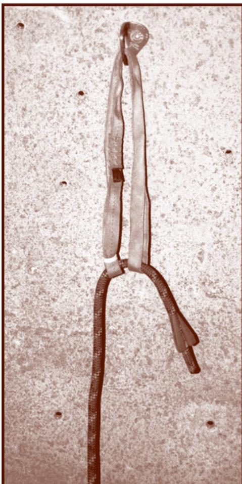
Figure 4—The Geartriever can recover slings and runners. A sling is passed through a fixed anchor. The Geartriever is attached to the end of the climbing rope. A tension band is placed on one end of the sling. When the rope is pulled, the sling comes with it.
