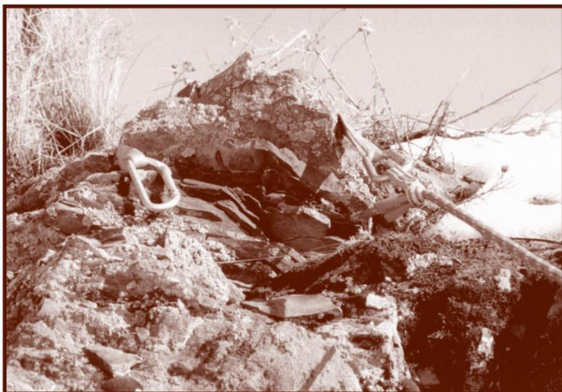
Figure 5b—The Geartriever is pulling a sling and carabiners from a rock horn.
