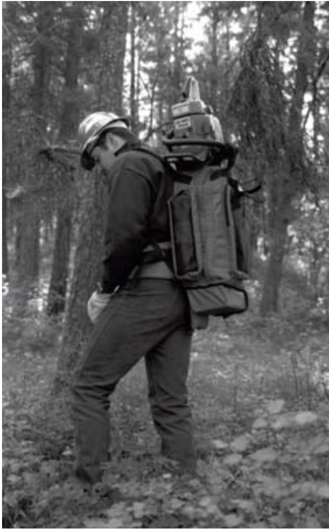
Figure 2b—Epperson Mountaineering chain saw pack (side view).
