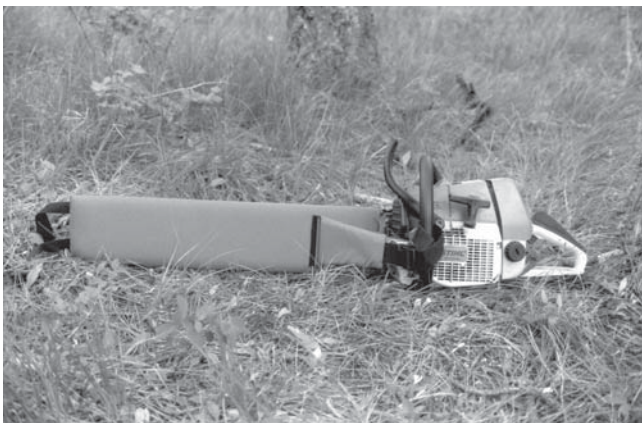
Figure 3—Chain saw bar in removable sleeve of the Epperson Mountaineering chain saw backpack.
