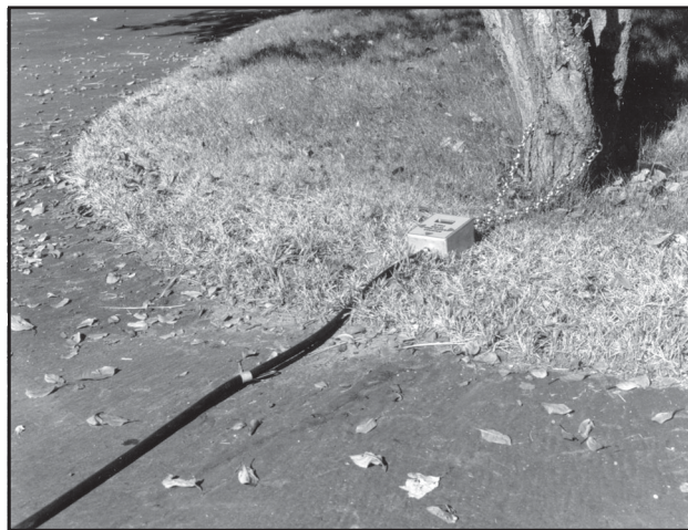
The K-Hill KBA-II pneumatic counter is one of the two types of counters being supplied to Forest Service field units by MTDC.
