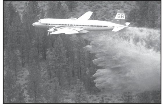
*The Forest Service program that tests airtankers is being moved to the San Dimas Technology and Development Center. This photo shows Tanker 66, a DC-7, using an Aero Union retardant delivery system.*
