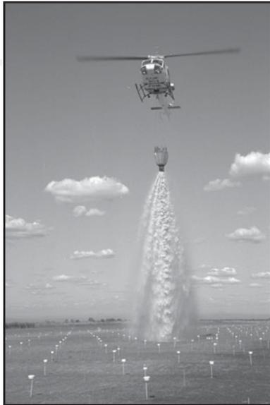
Tests using a field of cups arranged in a grid reveal the pattern of deposition for fire-retarding chemicals dropped from aircraft.
