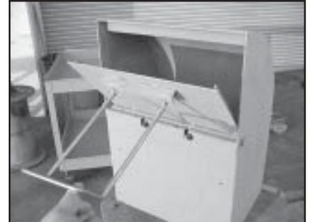
The swing handle on this bearproof refuse container is easily opened with one finger.
