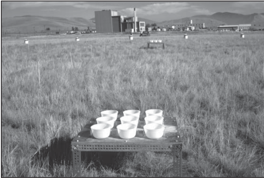
Figure 11—Table of nine cups for measuring variation around a single sample point.
