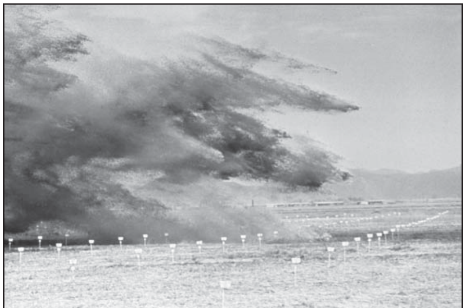
Figure 12—An example of retardant reaching the ground before forward momentum has stopped.
