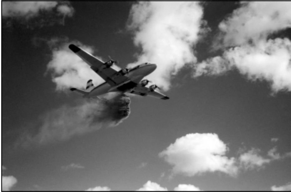
Figure 7—Gum-thickened retardant dropped by the Aero Flite DC-4 airtanker.
