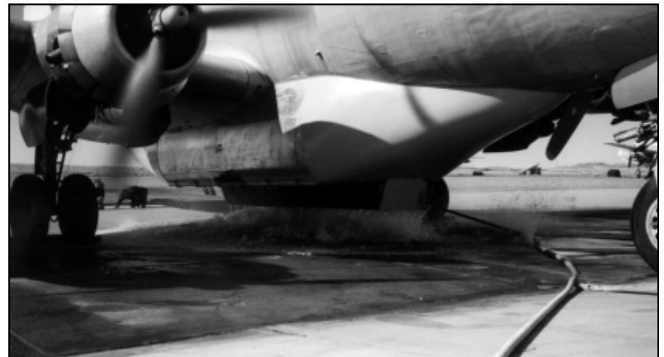
Figure 1—A static test of the Aero Flite DC-4 airtanker.
