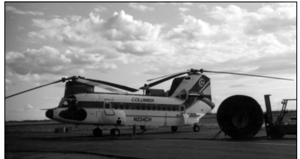
Figure 1—The Columbia BV-234 using the modified 3000-gallon Griffith helibucket.
