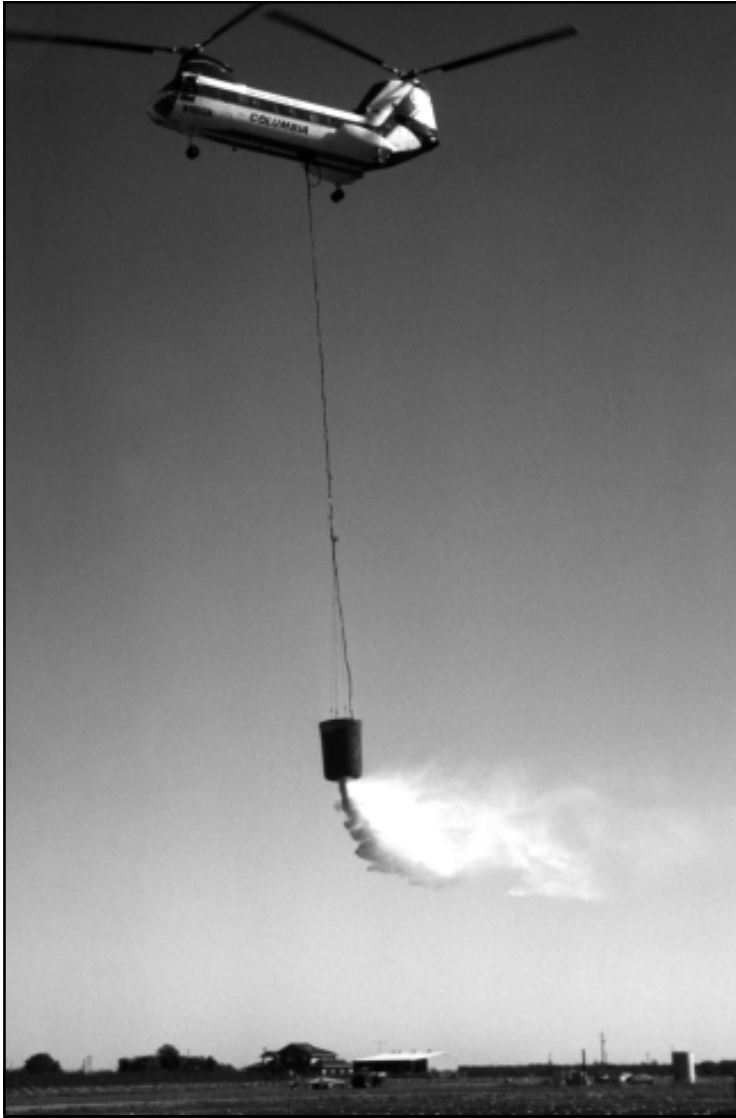
Figure 8—Drop test of the Columbia BV-107 helicopter using the 1000-gallon Griffith helibucket to drop gum-thickened retardant.
