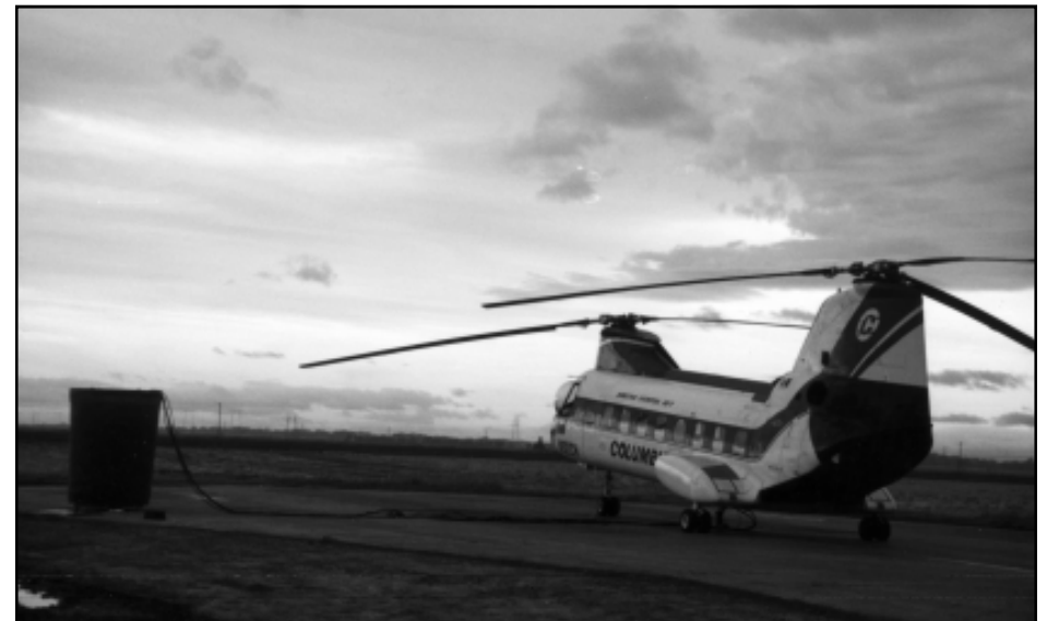
Figure 1—Columbia BV-107 helicopter using the 1000-gallon Griffith helibucket.
