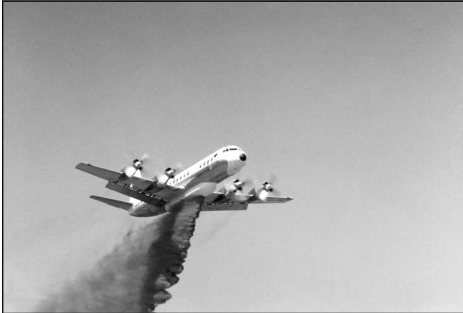
Figure 6—Drop test of the Airspray Electra L-188.
