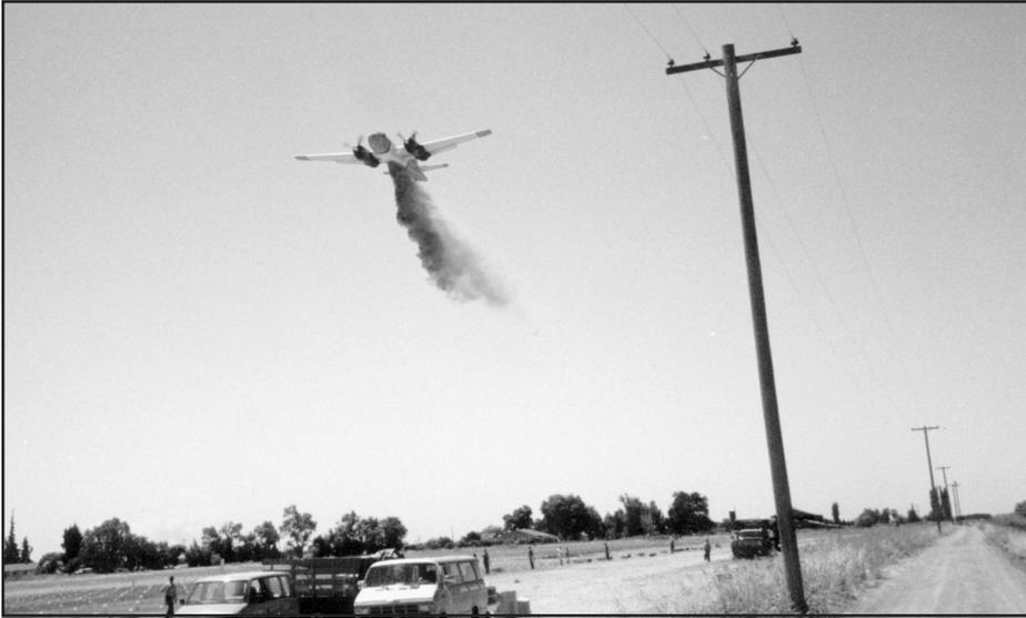
Figure 6–Drop test of the Aero Union SP-2H.
