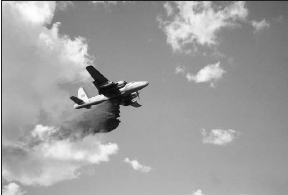
Figure 7—Gum-thickened retardant being dropped by the Neptune P2V-7.
