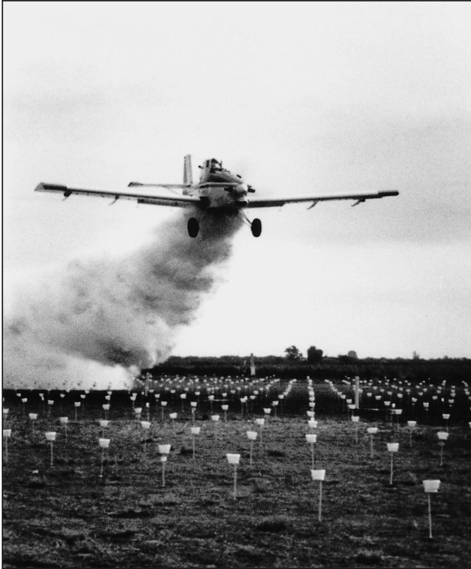
Figure 3—Drop test of the Ayres Turbo Thrush.
