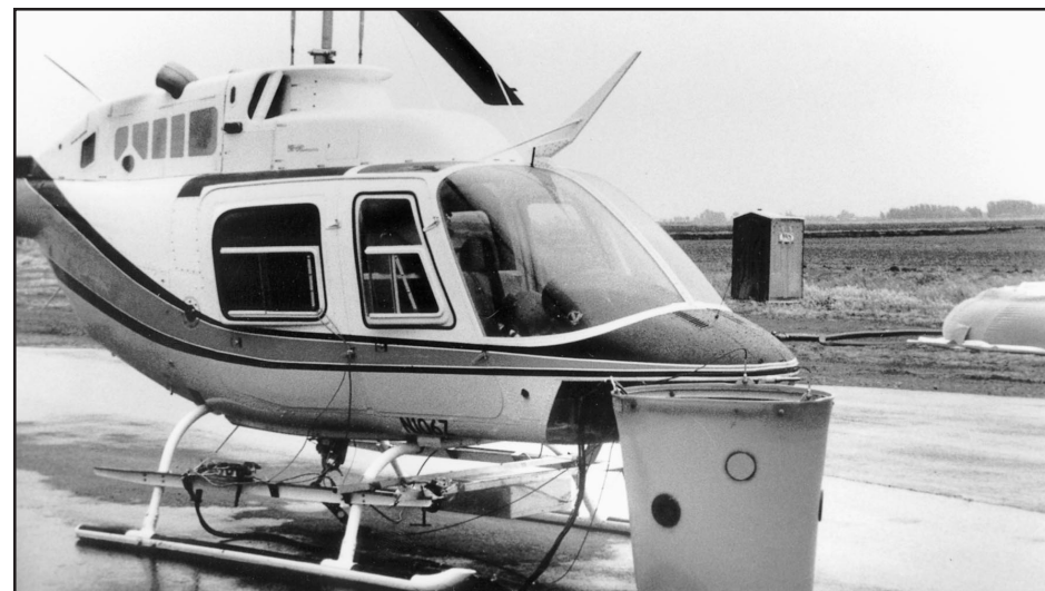
Figure—1 Griffith 100-gallon helibucket.
