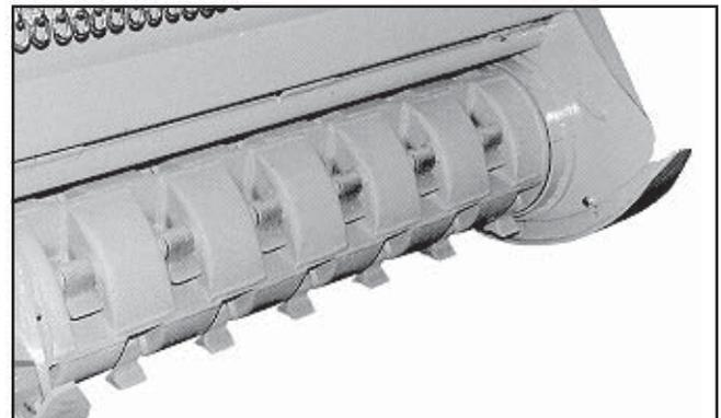
Figure 4—Seppi M drum shredder with free-swinging cutters.
