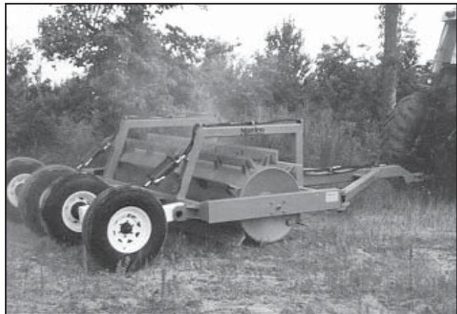
Figure 2—Rolling chopper used for land clearing.
