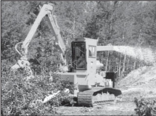
Figure 8—Track Bandit Model 1900 self-propelled whole-tree chipper.
