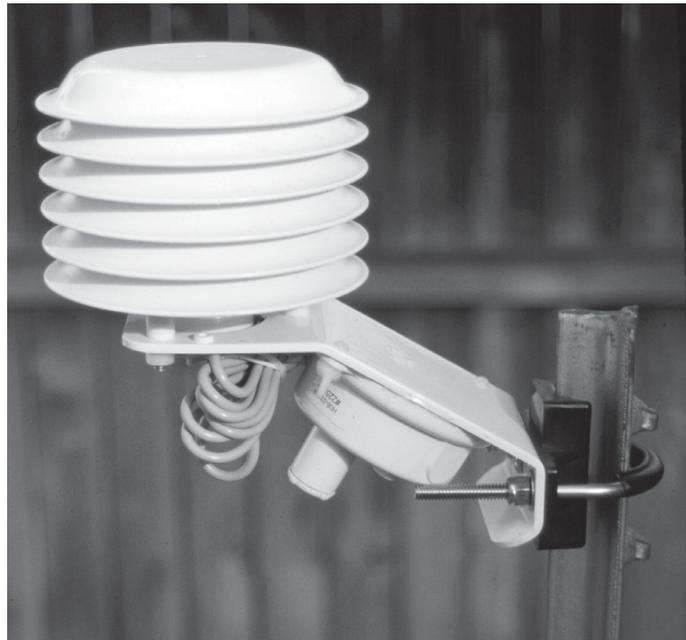
Figure 2—The radiation shield's U-bolts were used to mount the HOBO data logger on a metal fence post. The radiation shield is in the normal operating position.
